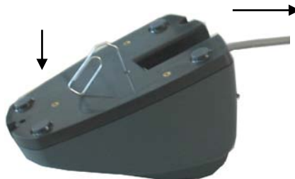
Disconnecting the Cable
